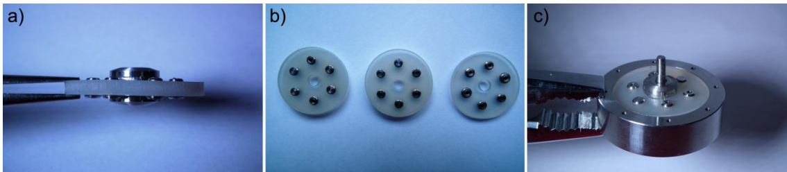
Figure III.6. Picture of the silicone membrane. a) Lateral view. b) Three possible configurations; from the left: 2, 4 or 6 open holes, respectively. c) Silicone membrane assembled with the check valve system.
