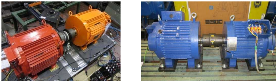
Figure 10.15 – Test motors identified at a stabilized temperature level. a) FASR prototypes presented in Chapter 08. b) Other motors for elevator with a Surface Mounted PM rotor configuration
