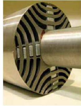
Figure 11.6 - Rotor lamination of the motor under test, whose main data are listed in Table 11-I.
