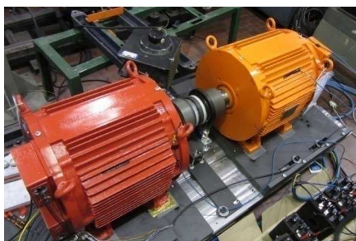
Figure 8.5 - Two FASR “twin” prototypes, shaft connected on the test rig. A torque-meter is interposed between the two motors.
