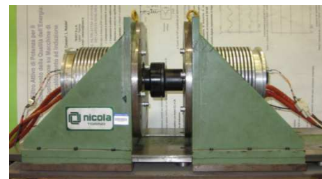
Figure 10.10 - "Twin" traction PM Assisted Synchronous Reluctance motors, shaft connected and controlled by power converters having the dc-link in common.
