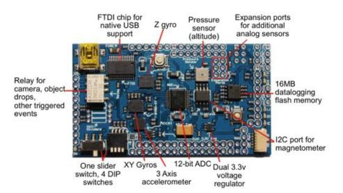
Figure 4.2: The OilPan Inertial Measurement Unit
