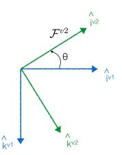
Figure 2.7: The vehicle-2 frame. If the roll angle is zero, then the x axis points out the nose of the airframe, the y-axis points out the right and the z axis points out the belly
