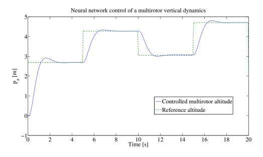
Figure 10.20: Neural network controlled vertical position
