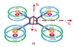
Figure 1.19: Octorotor X flight and design configuration
