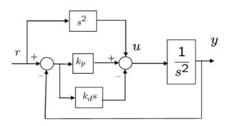
Figure 8.4: Feedforward term is added to a standard PD loop
