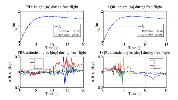
Figure 9.10: PID and LQR controlled height and attitude angles during free flight
