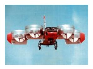
Figure 1.5: Bell X-22 Ducted Fan Research Vehicle
