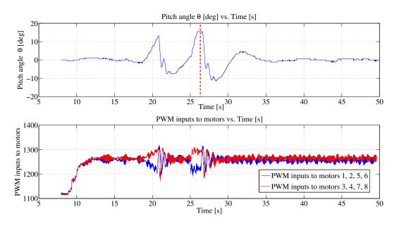
Figure 9.8: Experimental PID controlled pitch output and relevant motors inputs
