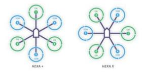
Figure 1.15: Hexarotor + and X flight configurations
