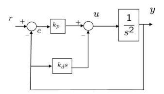
Figure 8.3: Standard PD loop
