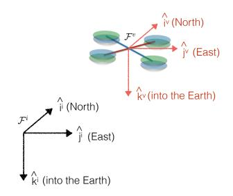
Figure 2.5: The vehicle coordinate frame. The x-axis points North, the y-axis points East and the z-axis points into the earth
