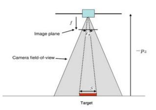
Figure 8.1: The size of the target is S in meters and the size of the target in the image plane is denoted by  $\epsilon_s$  in pixels. The focal length is f and the height above the target is  $-p_z$
