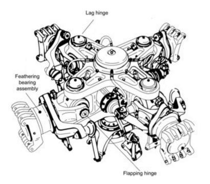
Figure 1.1: Full-scale helicopter swashplate [1]
