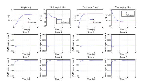
Figure 9.2: Nonlinear dynamics of a LQ regulated aggressive maneuver; the rotors position in the figure recalls the physical rotors position in the multirotor
