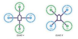
Figure 1.14: Quadrotor + and X flight configurations
