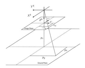
Figure 6.1: Camera model for the multirotor
