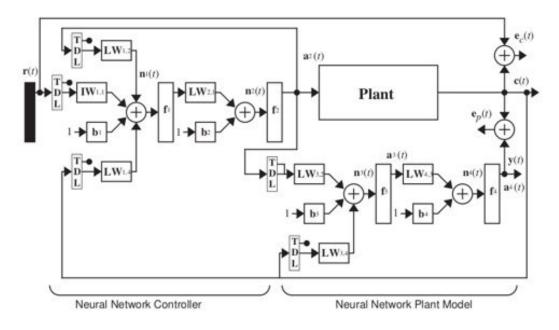
Figure 10.17: Detailed model reference control structure
