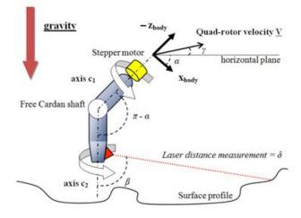
Figure 10.22: Distance sensor embodiment
