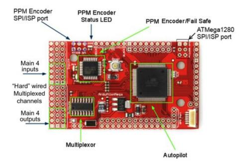
Figure 4.1: The Ardupilot Mega board
