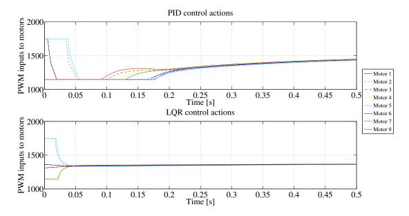
Figure 9.4: Control actions: PID vs. LQR
