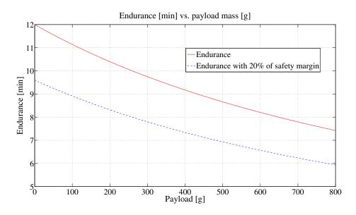
Figure 4.4: Multirotor endurance as a function of the payload mass
