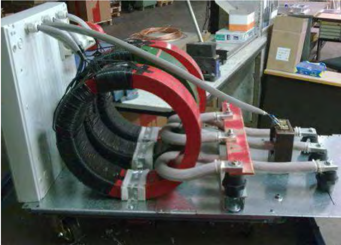
Figure 21 Image of the iron core and of the primary and secondary windings
