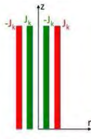
Figure 5 Representation of the column of a transformer by means of two solenoids rectangular section
