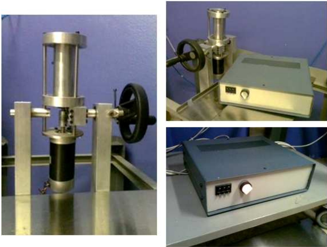
Figure 3.7: Rotational casting equipment used for the cladding tubes fabrication
