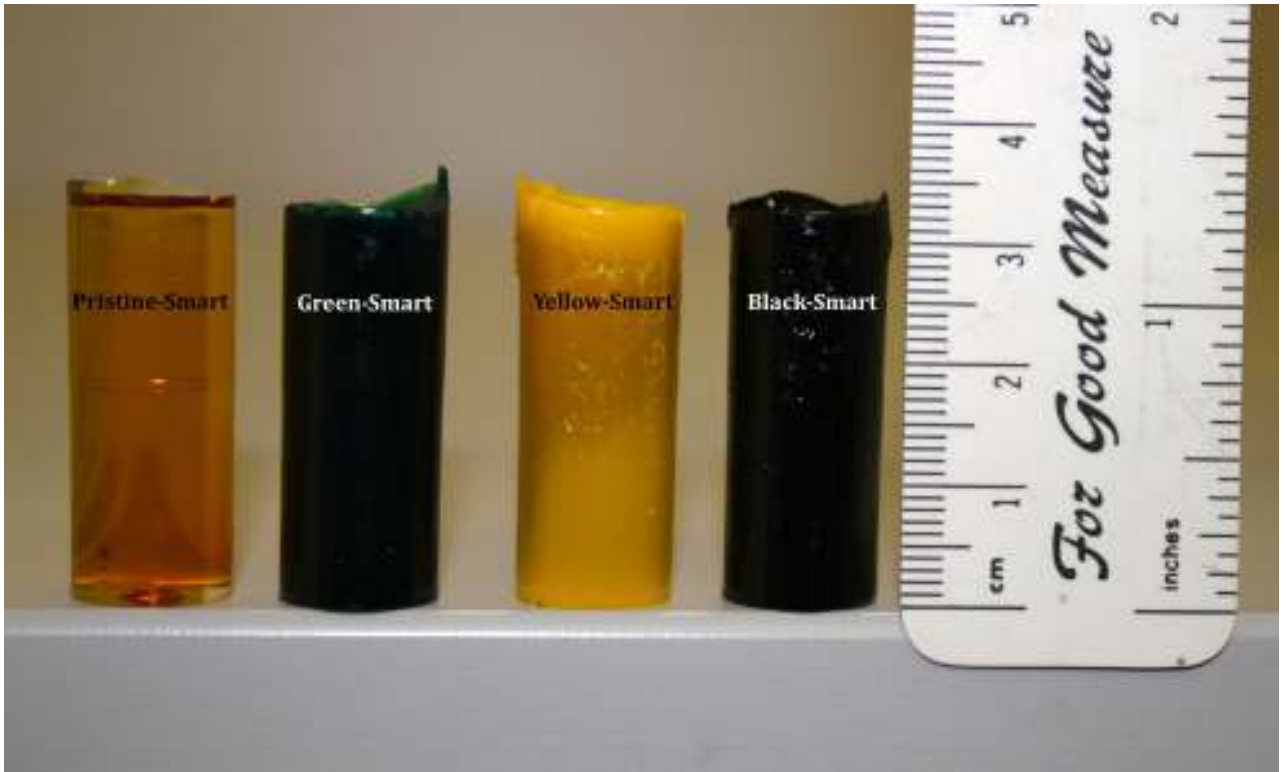
Figure 4.49: 30mm Thick Pristine and Colored Samples
