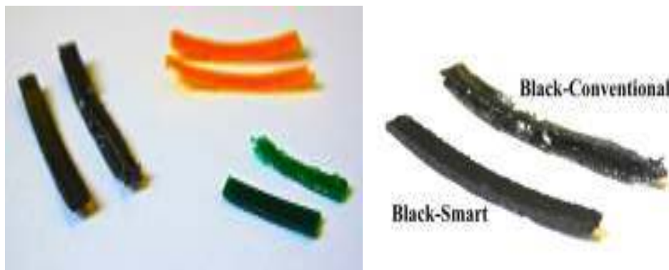
Figure 4.44: 1mm thick colored epoxy samples
