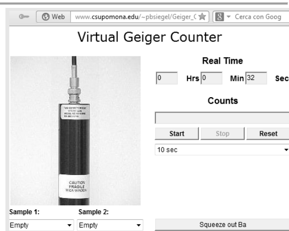
Figure 3 - Screenshot of the virtual laboratory of radioactivity [11], equipped with a Geiger counter and two sample holders. These holders can be left empty to measure the natural background, or loaded with two different types of radioactive sources.
