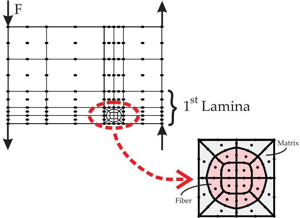
Figure 4.17. Laminate beam structure with one fiber/matrix cell included under torsion loading.
