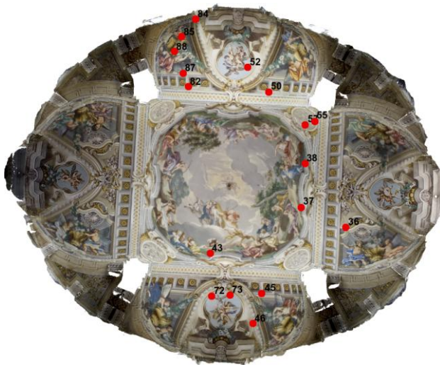
Figure 5 GCP used for bundle block adjustment
