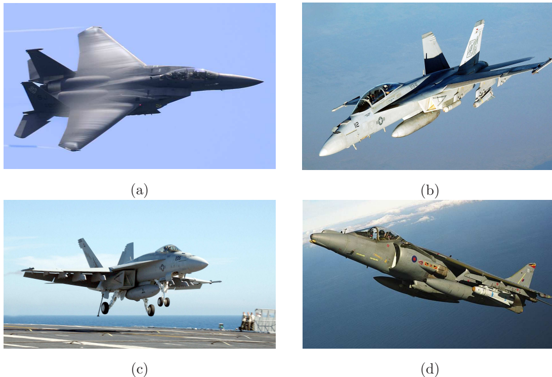
Figure 1.1. Utilisation of composite material in military airplanes: (a) F-15 (early 1970s), 2% composites, (b) F/A-18 A/B (mid-1970s), 10% composites, (c) AV-8B Harrier (early 1980s), 27% composites, (d) F/A-18 E/F (mid-1990s), 22% composites.
