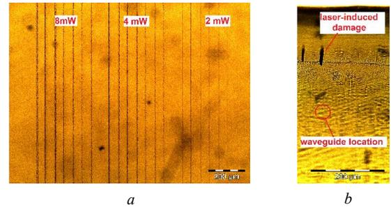
**Fig. 1** Microscope images of waveguides written at 8, 4 and 2 mW: a) top view and b) cross-section view. The artefact in b) indicates the location of a waveguide,  $300\text{ }\mu\text{m}$  below the surface. Close to the surface, the damages produced by the FS laser are visible as dark vertical lines.
