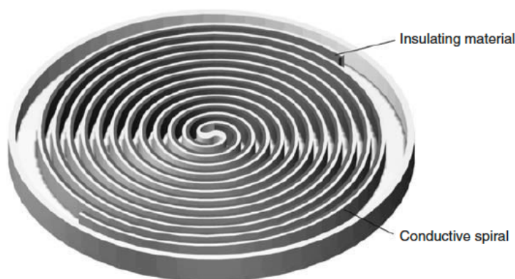
Figure 13: The structure of the spinning disc heat transfer surface. Overall heat transfer coefficient of 10 \text{ kW/m}^2 \text{ K} for low viscosity process fluids and water or glycol as heat/cool fluid. A 0.5 m dia disc with \Delta T 20 K will transfer 39 kW, thanks to patented double spiral disc design, copper construction (with chrome plating for corrosion resistance)
