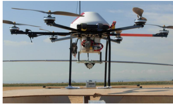
Figure 3 The Microkopter hexacopter modified by RESTART
