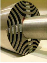
Figure 6. Rotor lamination of the motor under test
