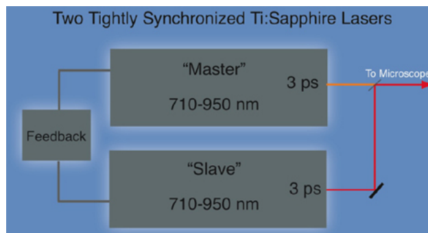
Fig. 2.7 Scheme of two mode-locked synchronized lasers.
