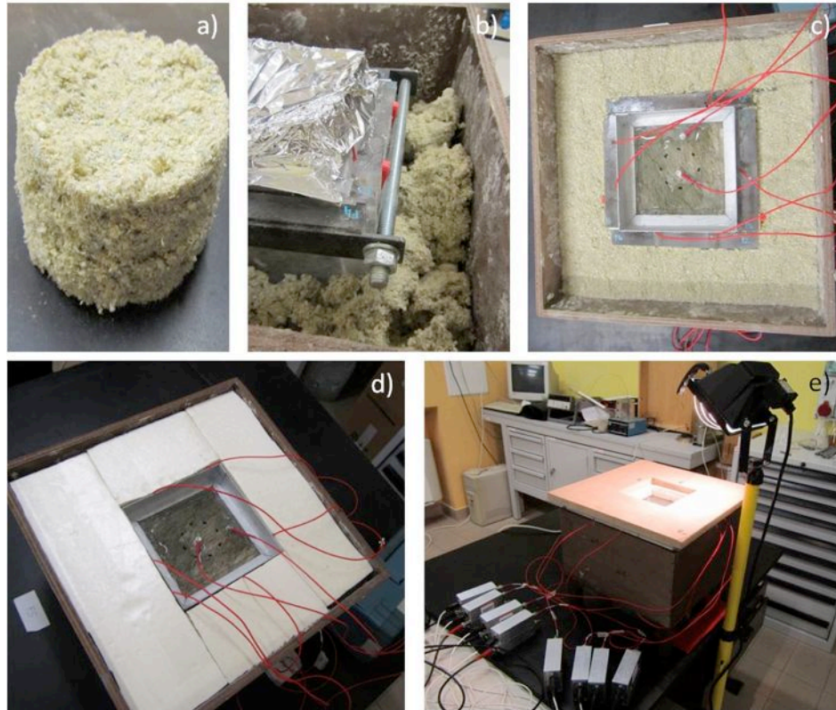
Figure 8.10: Thermal insulation: a) sample of cellulose fiber provided by Nesocell; b) cellulose fiber compacted in the wooden box; c) stainless quadratic pool glued on the top of the specimen; d) 8cm thick polystyrene sheets around the pool; e) transparent plexiglass, MDF sheets and IR lamp installation.
