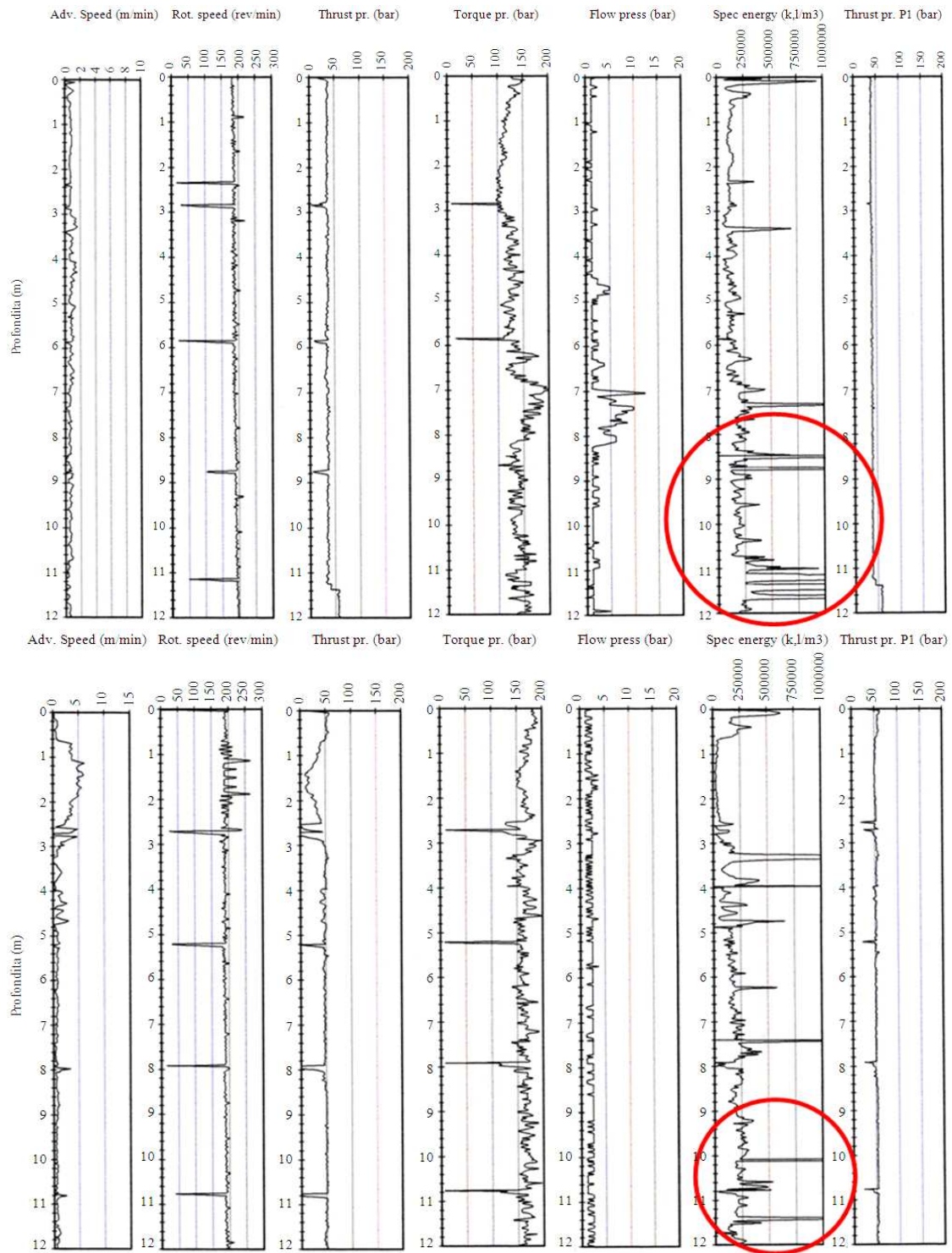
Fig. 1. Diagraphies D1-D3 of the drilling parameters recently realized in the subsoil of Turin: red circles indicate the increase of the specific energy due to cemented layers
