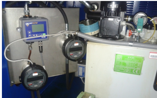
Figure 1: Inline contamination monitor connected to the lubrication system of the splined couplings test rig.
