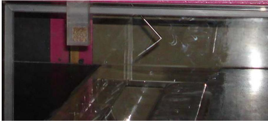
Figure 2.8. Detail of the hot wire probe holder. Flow is from left to right.
