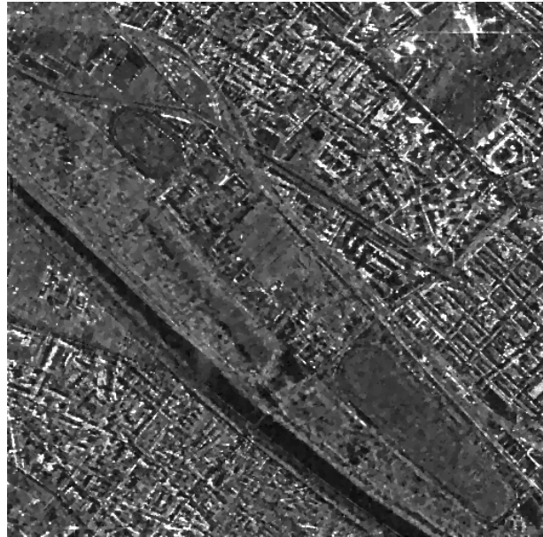
Fig. 12. Example of the application of the TV filter in [122] to the 4-look COSMO-SkyMed image in Fig. 10-(a).
