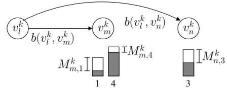
Fig. 6. Greedy relaying example. In phase 1, downloaders  $v_m$  and  $v_n$  have incomplete content 1, 4 and 3, respectively, and announce the missing data. In phase 2, relay  $v_l$ , storing all missing data, allocates its airtime to satisfy the requests by  $v_m$  and  $v_n$ , adopting a water-filling approach.
