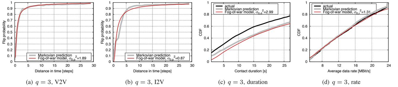
Fig. 3. Flip probability predicted through third-order Markovian chain, for V2V (a) and I2V (b) contacts; the corresponding values of  $\sigma_{0,p}^2$  are also reported. CDF of the contact duration (c) and data rate (d) for the third-order Markovian chain prediction, with corresponding values of  $\sigma_{0,d}^2$ ,  $\sigma_{0,r}^2$ .
