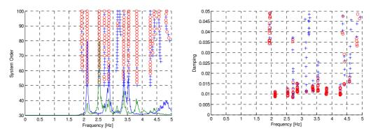
Figure 5: Stabilisation diagram: o stable modes + unstable modes —AT3X —AT3X Stabilisation criteria: 1% Frequency, 5% Damping, 2% MAC.
