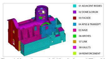
Figure 4: Macro-elements subdividing the damaged FE model.
