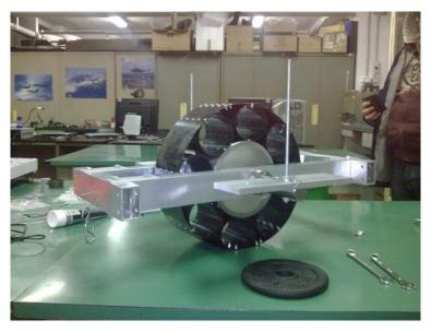
Figure 96 A structural similitude model: the "scaled wheel"
