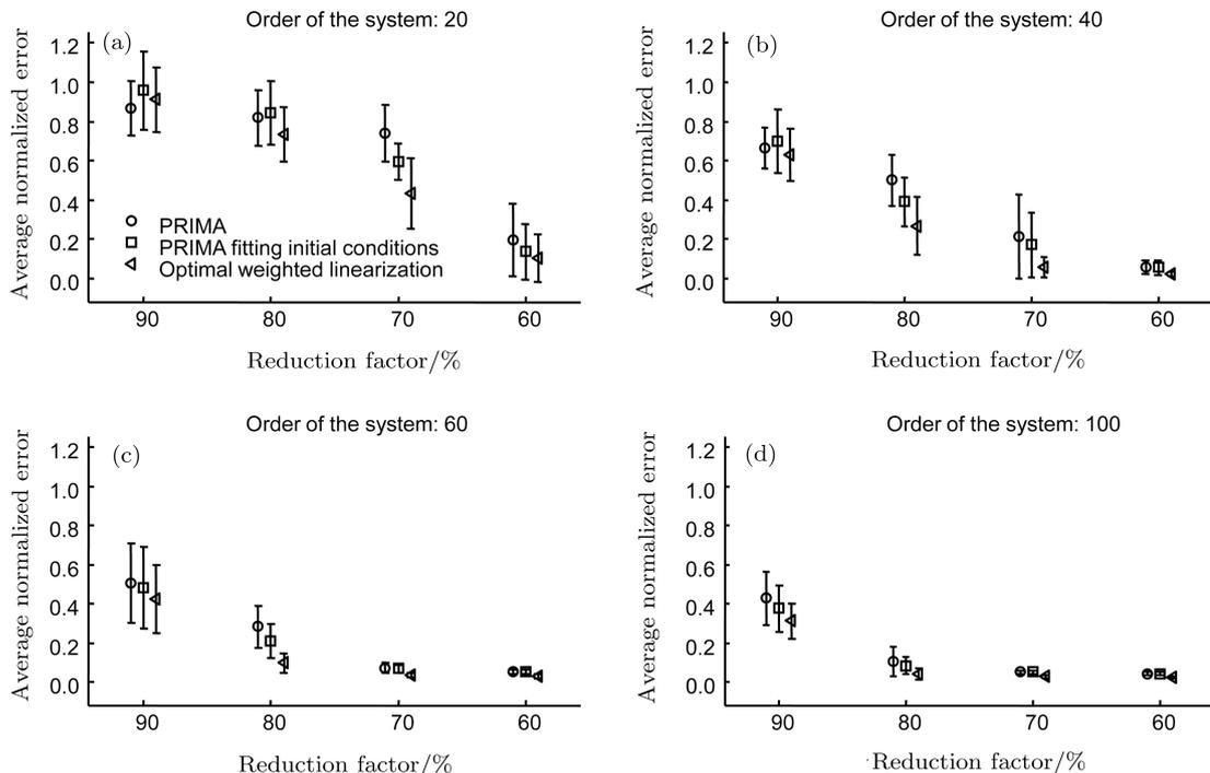
**Fig. 5** Average error in approximating different systems of equations, using different methods (standard PRIMA, PRIMA fitting initial conditions, optimal reduction including additional weighted linearization of quadratic term) and with different reduction factors. The order of the complete systems are (a) 20, (b) 40, (c) 60, and (d) 100. Mean and standard deviation of errors over 10 repetitions are shown.
