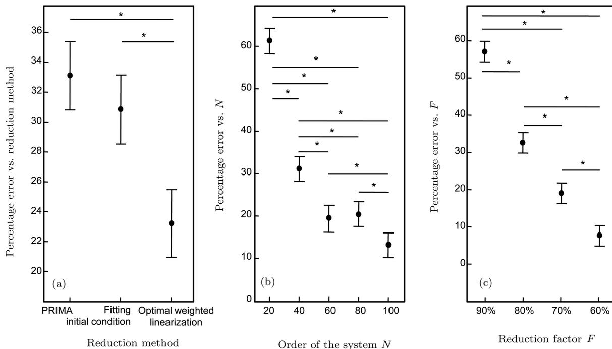
**Fig. 6** Statistical analysis of the average error as a function of three factors: (a) Reduction method (standard PRIMA, PRIMA fitting initial conditions, optimal reduction including additional weighted linearization of quadratic term), (b) Dimension  $N$  of the system to be reduced and (c) Reduction factor  $F$ . Asterisks indicate highly significant differences ( $p < 0.001$ ).
