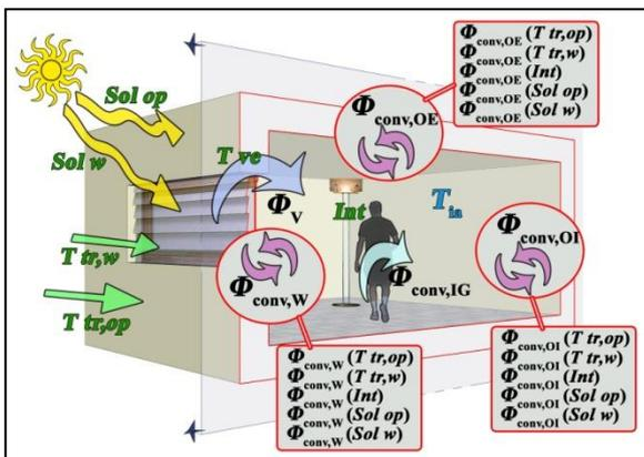
Fig. 1 – Driving forces and convective heat flows
