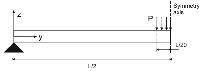
Figure 8: Simply supported beam under a localised uniform pressure P
