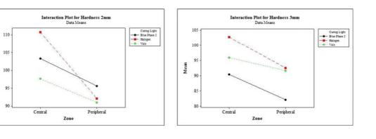
Conclusions: The tested hypothesis was rejected since none of the tested curing light produced a uniform micro-hardness distribution on nanofilled composites. In all cases, the peripheral area was significantly softer than the central area, in particular when the tip was 2 mm from the composite surface.
