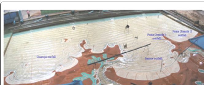
Figure 6: Scale model of Santos Bay, Estuary and Harbor and nearby beaches
