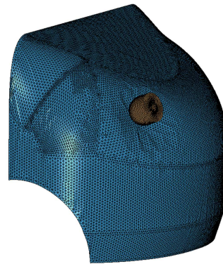
Figure 9. Impact test simulation for the frontal add-on.
