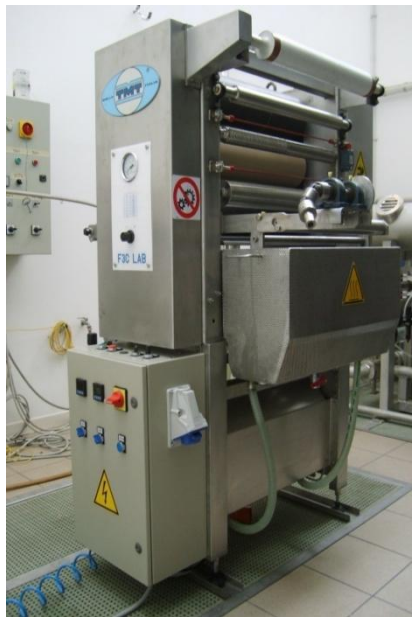
Figure 3.11 - Pad mangle machine used for squeezing fabric samples after the treatment.
