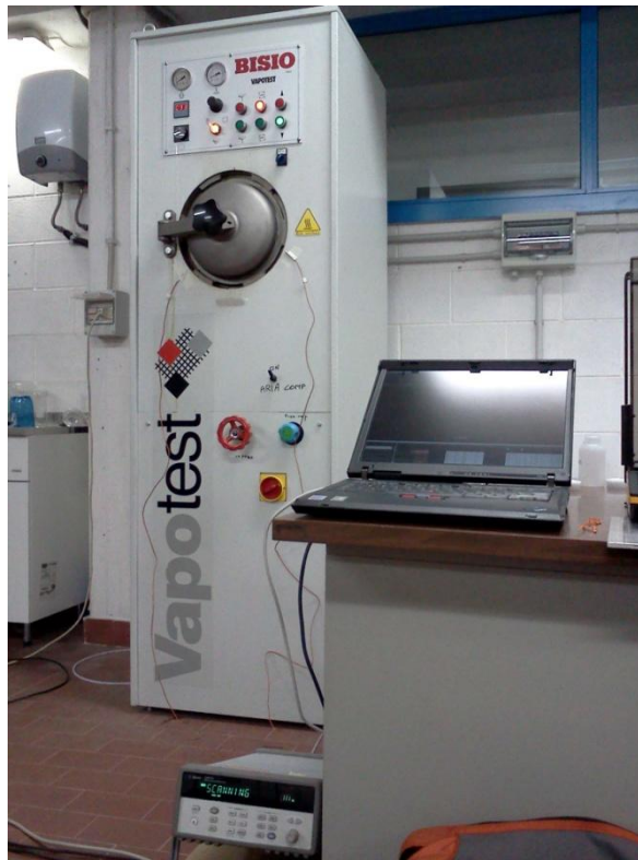
Figure 3.5 - Global view of the Bisio Vapotest equipment and the monitoring system.
