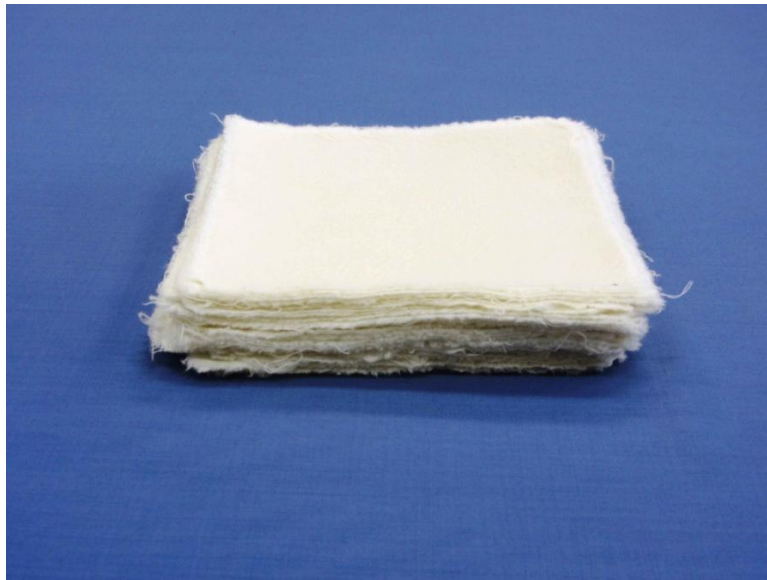
Figure 3.4 - Stack of fabrics constituting a 50 mm thickness bed.
