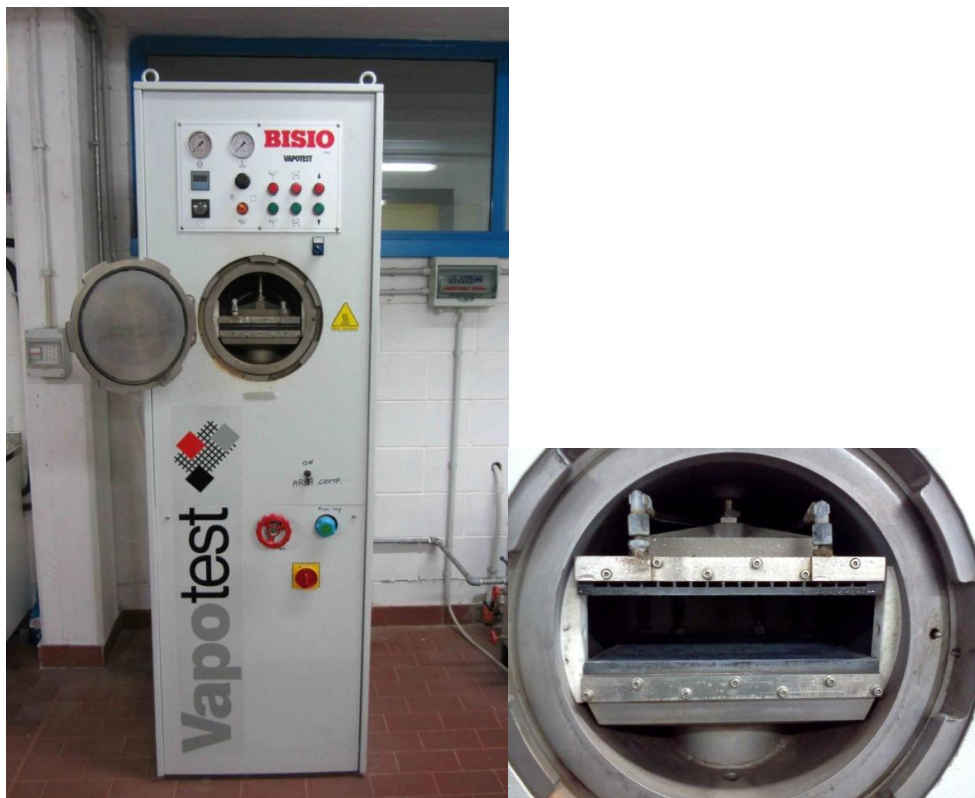
Figure 3.1 - Bisio Vapotest: front view (left) and detail of the treating chamber (right).
