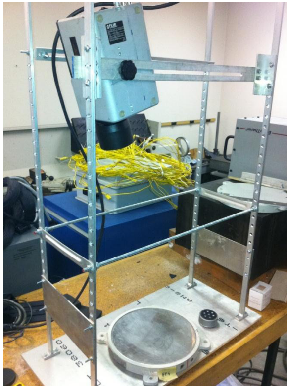
Figure 66: Thermo-camera SC 3000 used during pre-test on a scaled double pendulum bearing.
