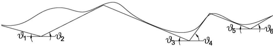
Figure 23: Schematic illustration of the roughness of sliding surface. Positive and negative \theta coexist.
