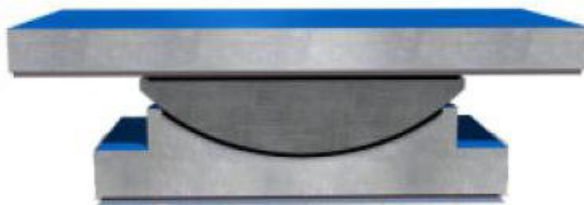
Figure 19: Sliding device with flat sliding surface.
