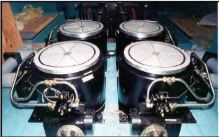
Figure 59: Four stationary hydrostatic sliding bearings/actuators, fixed to the concrete frame beneath the platen.
