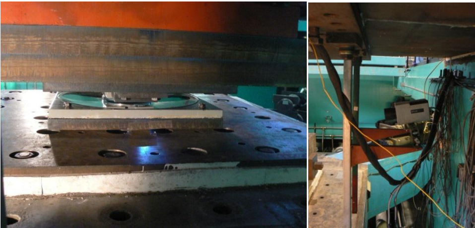
Figure 67: The left picture illustrates a field of view of the thermographic camera with the arrangement showed in the right picture.
