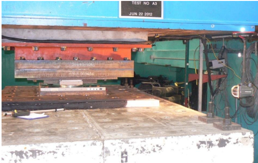
Figure 68: Final setup of the camera supported by a frame bolted to the bottom plate of the steel cross beam.
