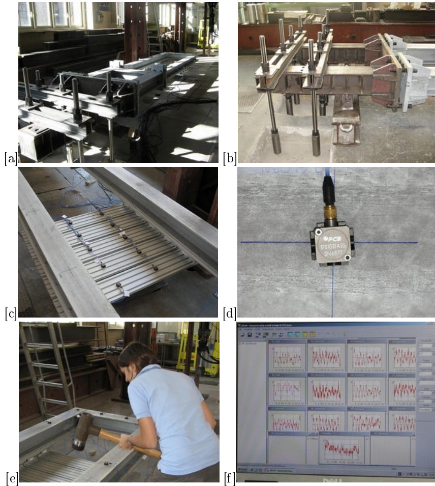
Figure 4.3: [a] The obstacle at the testing time in the “global” setup. [b] The supporting structure conceived as a joint. [c] Configuration example for the acquisition: the “plates” setup. [d] Accelerometer. [e] Instrumented hammer. [f] Screen shot taken during the acquisition time. Photos E. Bovet.
