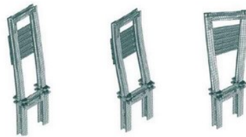
Figure 4.6: First three modes of vibrations, corresponding to the lowest frequencies, obtained through a numerical simulation in ADINA, from [21].
