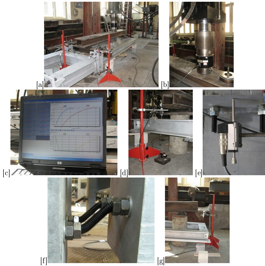
Figure 4.7: [a] The static test set-up. [b] Oleodynamic actuator. [c] Screen shot taken during the acquisition time. [d] Displacement transducers. [e] Particular of a displacement transducer. [f] Example of the deformed steel bars. [g] Final displacement of the obstacle tip. Photos E. Bovet.
