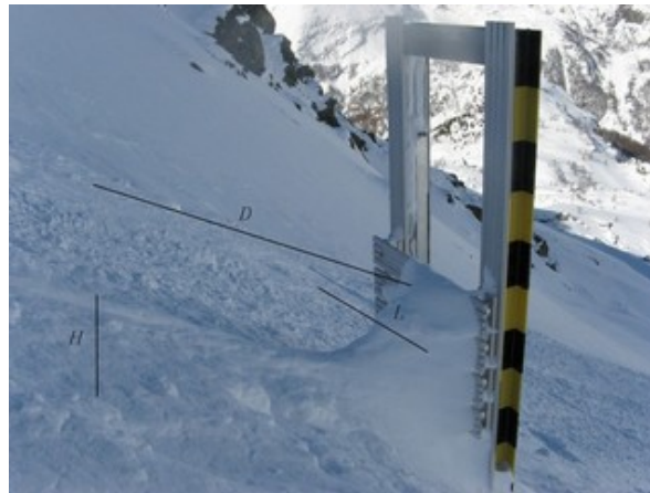
Figure 4.18: Height H of the snowcover, width L of the shape left upwards the obstacle and distance D along the slope from the obstacle.
