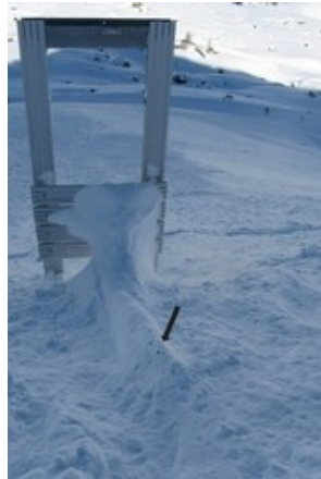
Figure 5.36: Shape of the snow upwards the obstacle after the avalanche of 5 th of March 2011. The black point is the place of the straw test A (see Sec. 5.1.2).
