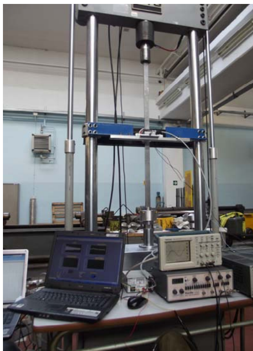
Figure 4.14 – A test on the rectified beam (specimen B1) for the evaluation of the natural fundamental frequencies under different imposed displacements.
