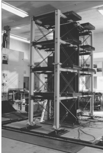
Figure 1.1 – A multi-degree-of-freedom hydraulic shaker used in testing civil engineering structures (University of British Columbia).
