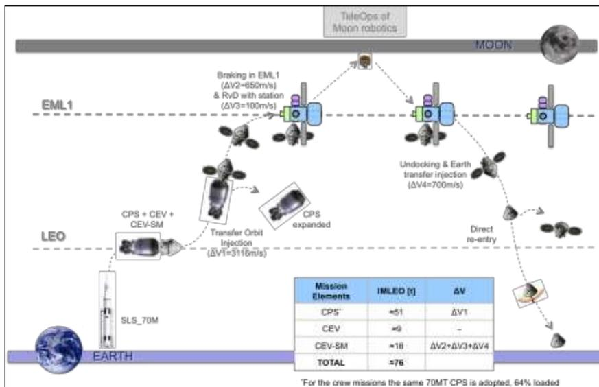
Fig. 9: Cis-Lunar Architecture – Crew Mission with Cryogenic Propulsion
