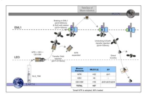
Fig. 10: Cis-Lunar Architecture – Crew Mission with Nuclear Propulsion
