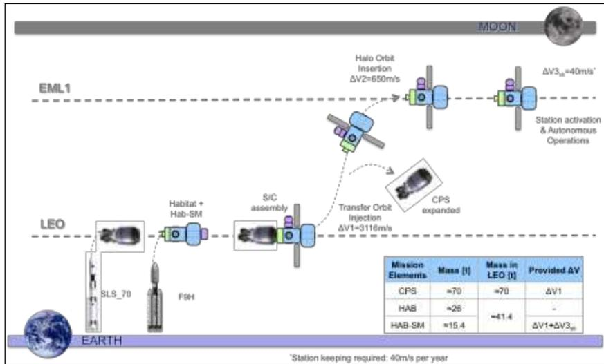
Fig. 8: Cis-Lunar Architecture – Cargo Delivery (EML1-HAB)
