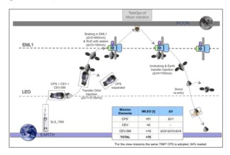
Fig. 9: Cis-Lunar Architecture – Crew Mission with Cryogenic Propulsion
