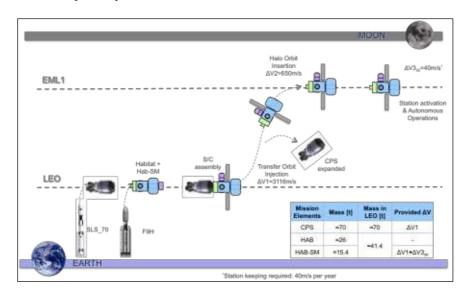
Fig. 8: Cis-Lunar Architecture - Cargo Delivery (EML1-HAB)
