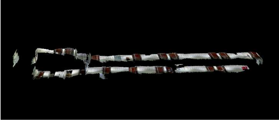
Figure 6.6: Top view of the long corridor experiment reconstructed using the presented plane-based SLAM. Note that it is more consistent and its shape is much close to the real scenario.
