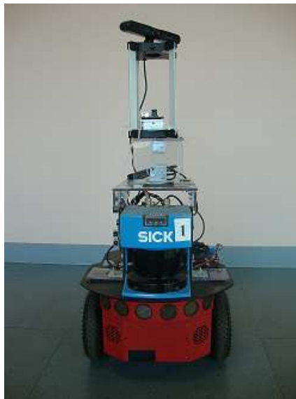
Figure 6.1: The robot used for the experiments is a differential-drive mobile robot equipped with a multitude of sensors: wheel encoders, a Sick LMS-200 laser range scanners and a Microsoft Kinect camera. As mentioned earlier in the text, only the wheel encoders and the Microsoft Kinect camera are used for this work. The laser scanner is only used for obstacle avoidance. For each frame, the Microsoft Kinect camera obtains 307,200 ( 640 \times 480 ) 3D points, corresponding to the dimension of the acquired image.
