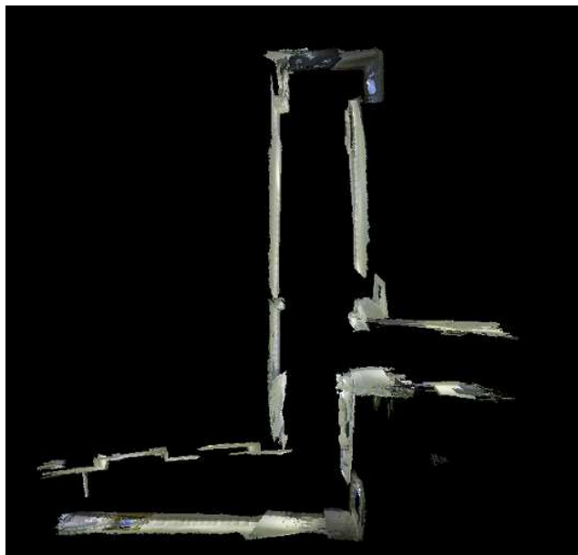
Figure 6.17: The 3D map constructed using plane-based SLAM. Its shape and orientation is much close to the real scenario. It clearly presents the main structures, e.g., walls, doors, pillars etc.
