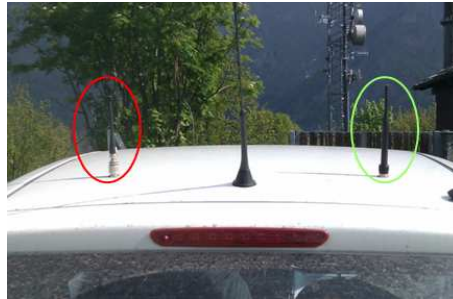
Figure 3.3: Antenna configuration on the testbed car: 700 MHz (red circle) and 5 GHz (green circle) antennas.
