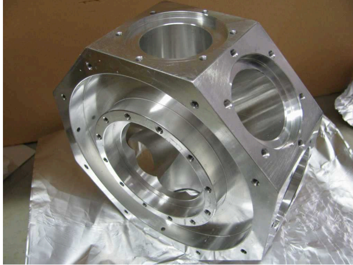
Figure 7.3: Picture of the custom aluminum chamber for the trapping region.
