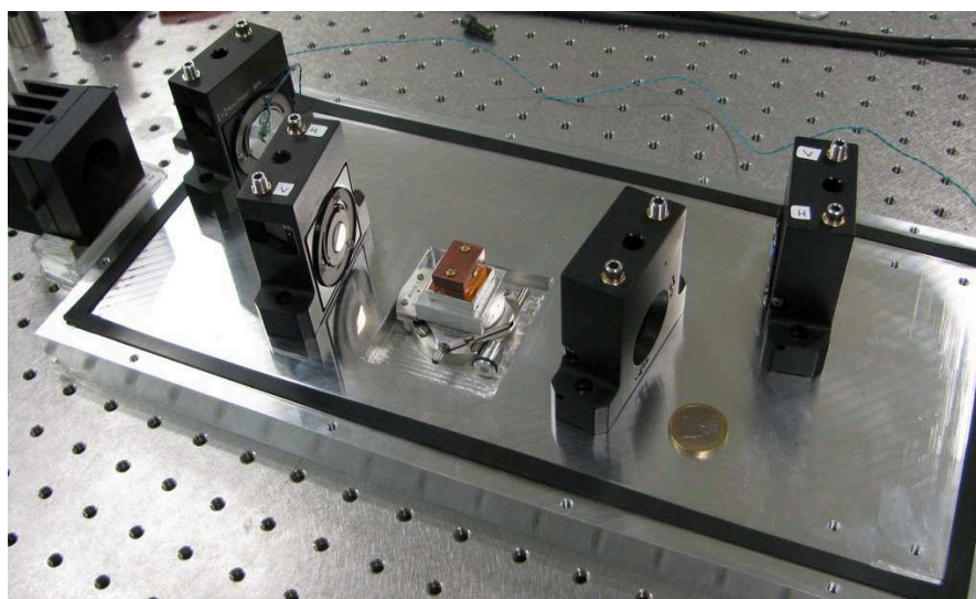
Figure 4.5: Picture of the cavity for the SHG of 399 nm. The LBO crystal is in the copper oven in the center.
