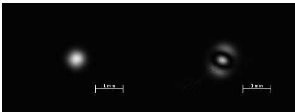
Figure 5.19: Transmitted cavity modes observed with a camera. Left, cavity well aligned in the TEM 00 mode; right, higher order mode with prevalence of the TEM 10 component.
