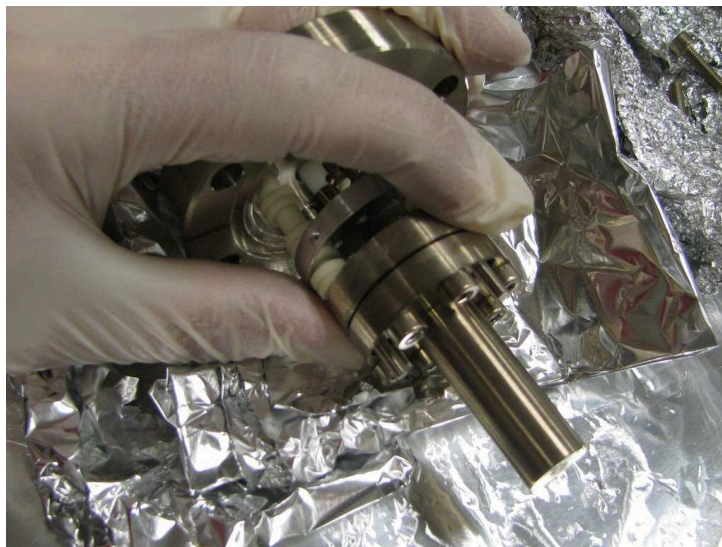
Figure 7.2: Picture of the atomic oven during assembling.
