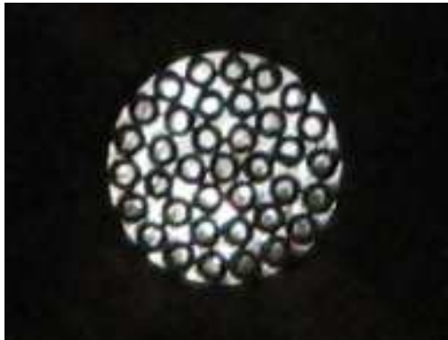
Figure 7.5: Details of the multichannel array. From this picture we can count 37 channels and 38 interstices.
