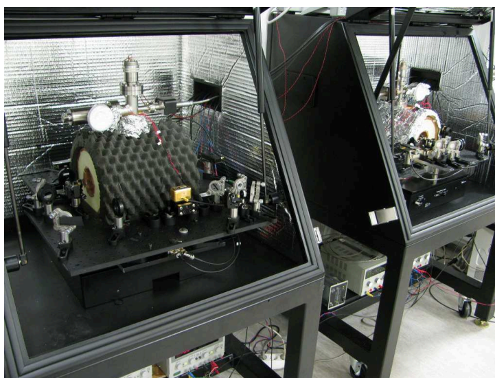
Figure 5.7: Picture of the two anti-acoustic chambers with the two setups for the ULE cavities.
