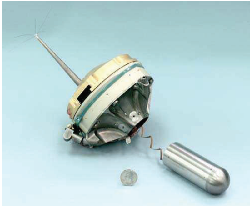
Figure 1.13: The disassembled parts of the Deep Space 2 probe, the forebody and the aftbody, as compared in size to a quarter. The two parts are linked by an umbilical (flexible interconnect).
