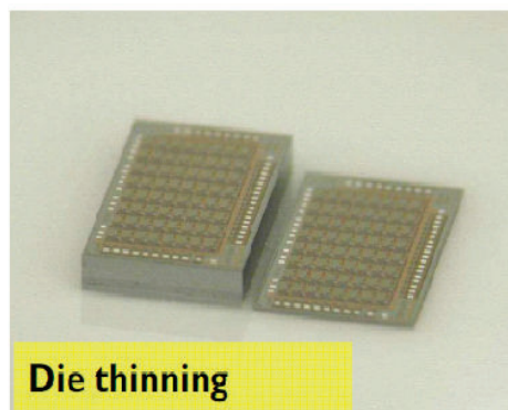
Figure 2.7: Wafer thinning example [78].
