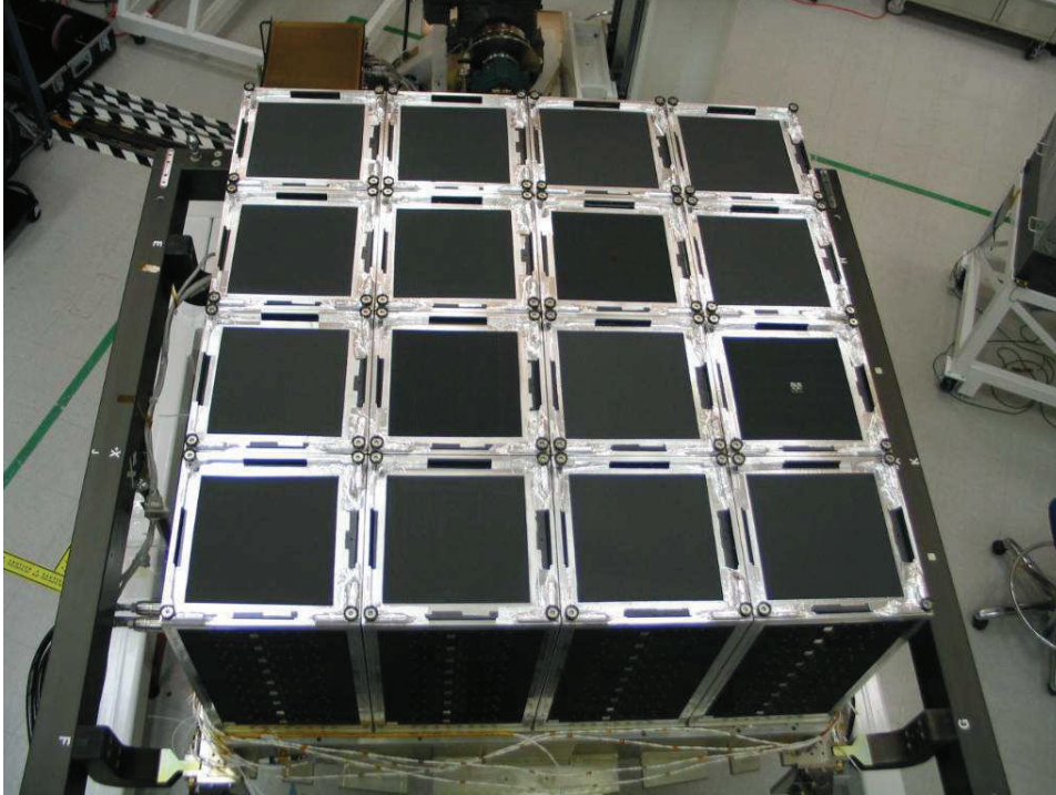
Figure 1.2: The GLAST tracking detector has nearly 900000 detector channels, each connected to its own amplifier. Packed into 16 compact modules are nearly 80 square meters of solid-state silicon detectors and 576 electronics boards, all supported on a carbon-composite structure.
