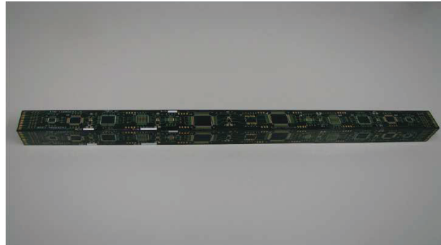
Figure 1.22: One of the box beam test articles assembled and ready for mechanical testing [65].
