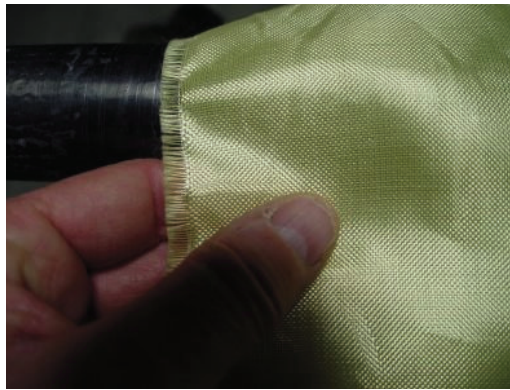
Figure 1.6: Lightweight (2.5 ounce/sq yd) bi-directional Kevlar cloth.
