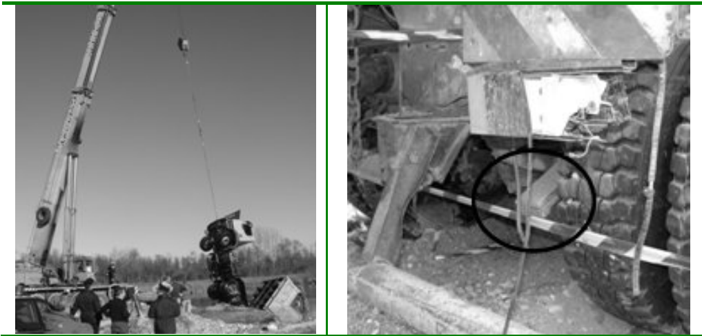
Figures 4.9 and 4.10: The recovery operations and the couple of collapsed leaf springs
