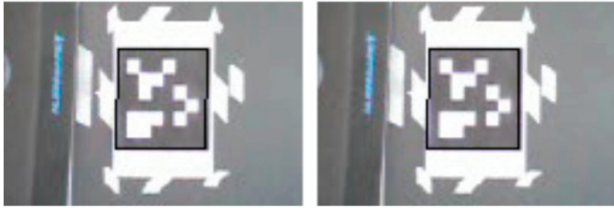
Figure 5. Pixel error: even in stable conditions, detected corners' positions might undergo discrete changes from frame to frame
