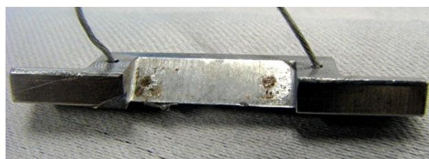
Fig.4.39 Wear trace on the flat surface of crossed curve-flat damper
