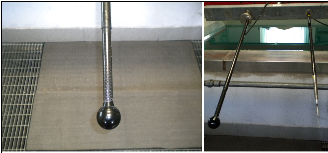
Fig 3.2.3.2 and 3.2.3.3. The transducer and the position of the hydrophone before of the immersion underwater.
