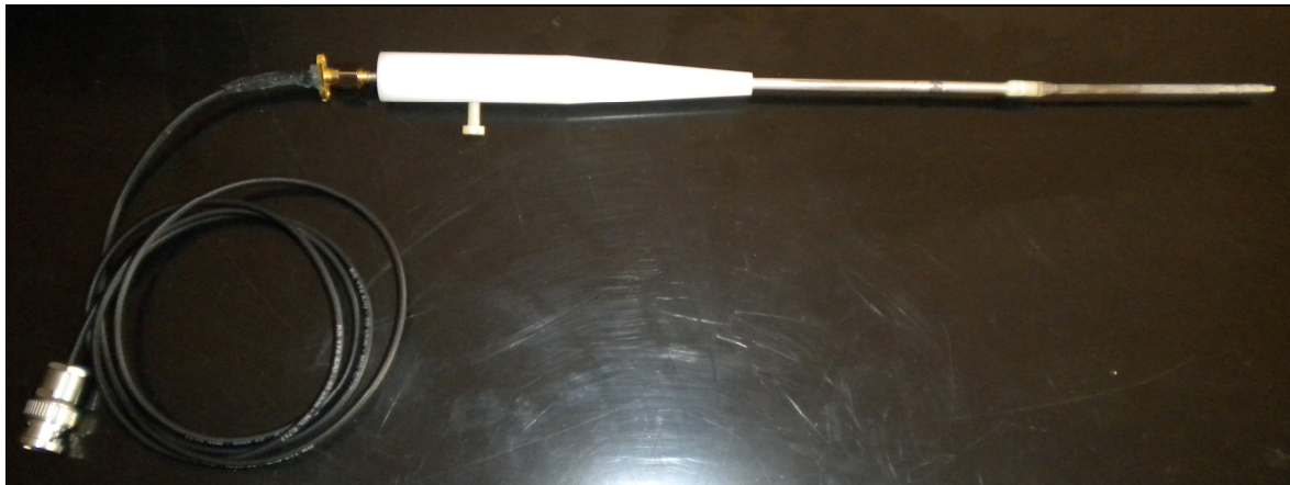
Fig 3.2.3.1. Hydrophone used for this work (from Acoustic Department of INRIM)
