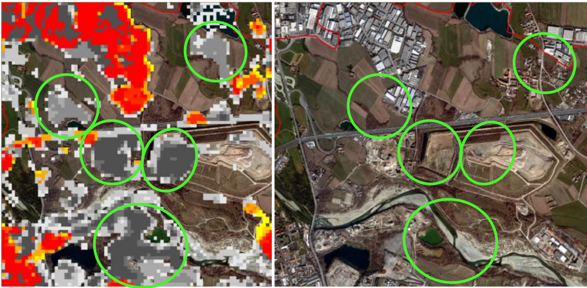
Figure 48 – Areas often incorrectly classified as urban: quarries or excavation site (lower circles) and cultivated fields (higher circles)
