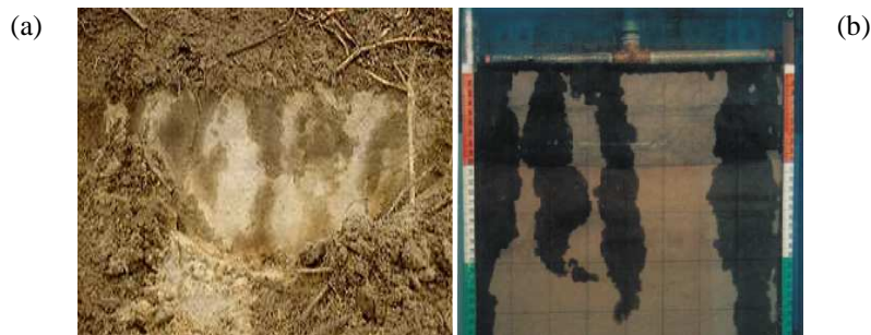
Fig. 68 – Preferential flow paths in water repellent soils (a) field image, http://www.splu.nl/waterrepellency ; (b) laboratory image, Doerr et al.(2000)
