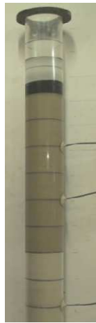
Fig. 22 – Column tests: soil moisture sensors positioning
