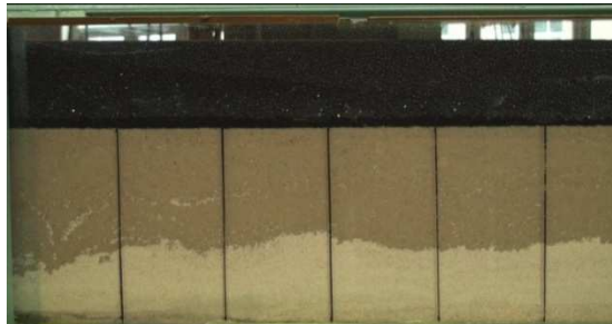
Fig. 8 – Sand “medium”, regicell 30/60 foam, pulse flow: instable infiltration flow during the depletion phase
