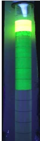
Fig. 20 – Column test: fluorescein dilution wetted the inner surface of the plexiglass column.
