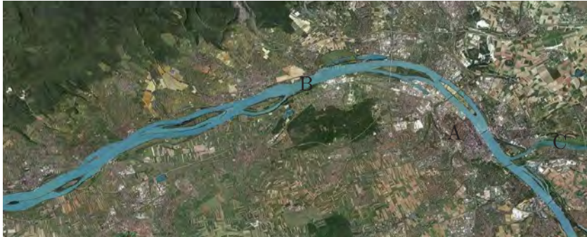
Figure 1.12. Navigation threatened by river morphological evolution, the case of the Rhine River: A Mainz, Germany; B Rhine River and; C Neckar River. The massive dunes formation begins in the reach just downstream of the confluence of the Neckar River in the Rhine River.
