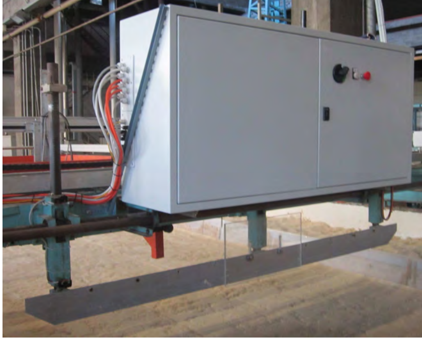
Figure A.4. Fixed steel blade and removable Plexiglas blade. In the picture a 50 cm wide Plexiglas blade is installed on the main blade.
