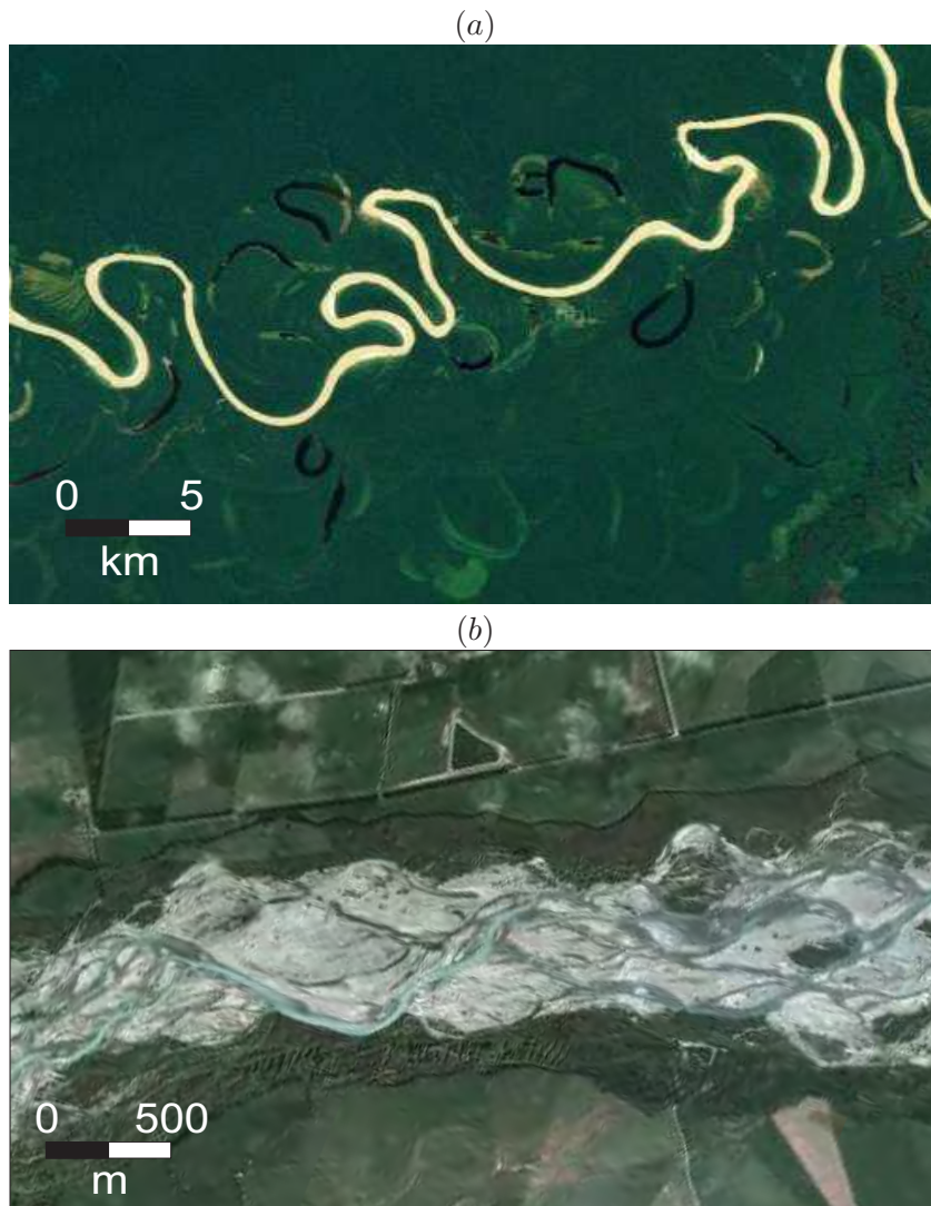
Figure 1.7. Examples of morphologies relevant for the planimetric evolution of rivers: (a) a meandering river and; (b) a braided river.
