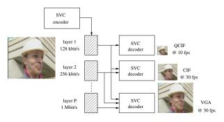
Fig. 5. Scalable video coding with P layers at increasing bit-rates. Decoding is done at different cumulative rates, yielding a video at increasing frame-rate and spatial resolution.
