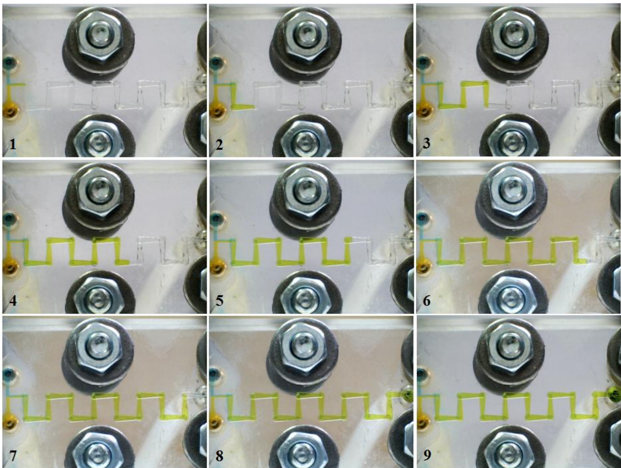
Figure 4.30 Chain 2-micromixer during the test at Re=0.416 .
