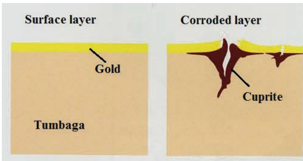
Figure 4: The gold-enriched layer is prone to cracking in the regions where there is more stress. Once the gold layer is breached, the copper in the underlying tumbaga becomes the reddish brown cuprite. Because the cuprite has a lower density than the surrounding alloy it swells outward and the depletion layer fractures and is forced away from the surface.
