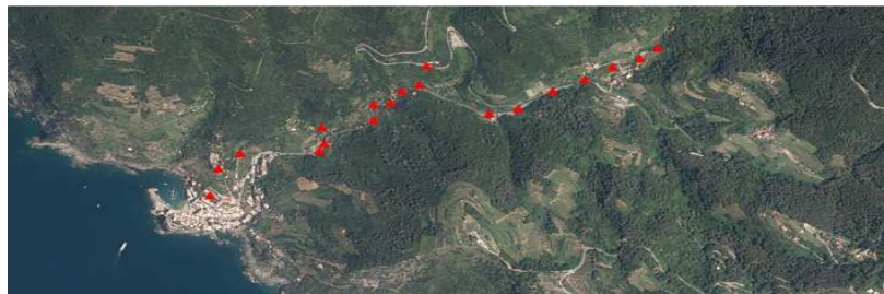
Figure 4: Location of vertices of the topographical network along the Vernazzola stream.
