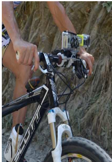
Figure 6: Mountain bike fitted with the stereo 3D go-pro cameras and a GPS receiver.
