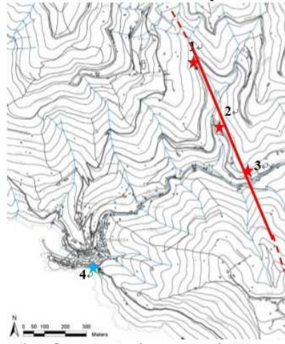
Figure 3: Location of geo-structural surveys on the Vernazza topographic map (1:5000), red line represents the major geological structure, the contact between the two formations Macigno and the Canetolo formations.
