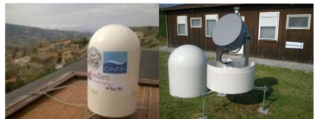
Figure 1. The X band mini radar with and without the radome.
